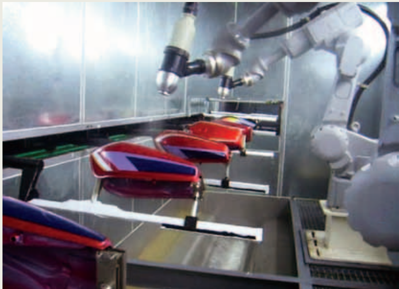
At a Chinese motorcycle producer, the motorcycle fuel tanks rotate as they travel through the coating booth
