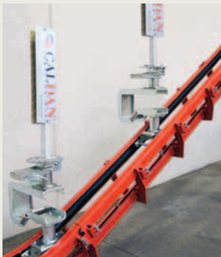
At a Chinese motorcycle producer, the motorcycle fuel tanks rotate as they travel through the coating booth
