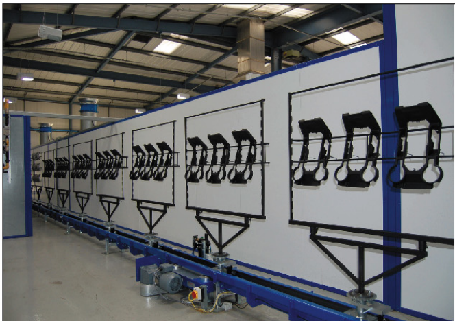
The paint line at M&S Automotive Coatings is based on a 121-metre long Caldan 'HD 100' floor conveyor system, which provides highly accurate positioning of the paint jigs and can operate on a batch "stop-go" or continuous basis, depending on production requirements. A floor-based system was selected in preference to an overhead conveyor as it minimises the risk of contamination of the parts — when coating plastics, optimum cleanliness is of paramount importance. Extremely stable and low in noise, the conveyor has a load capacity of up to 400kg per wagon and operates in temperatures of up to 250...C. It includes automatic lubrication to ensure smooth running, and also has the adaptability to be converted to power-and-free operation.
