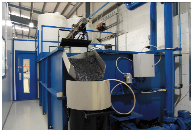
The parts are sprayed in a Delta 'Aqua-Flow' 5-metre modular water-wash spray booth by an ABB robot. The booth operates in conjunction with Delta's 'Aqua-Cleanse' sludge removal system, to form an integrated and highly cost-effective paint spraying and effluent treatment system. The Aqua-Cleanse unit removes 100% of the contaminated water from the booth and replaces it with clean, treated water, saving downtime and maintenance and enhancing the environmental impact of the paint plant.
