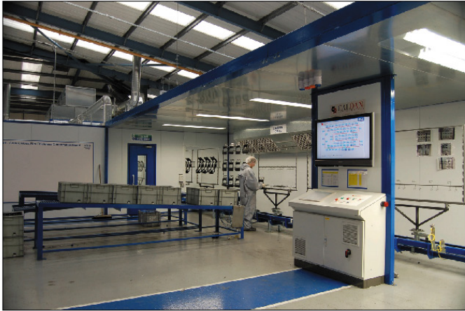
The parts are loaded manually onto rotating jigs and given a anti-static deionised air wash to remove dust. Positive air flow in the loading area also helps to minimise contamination.
