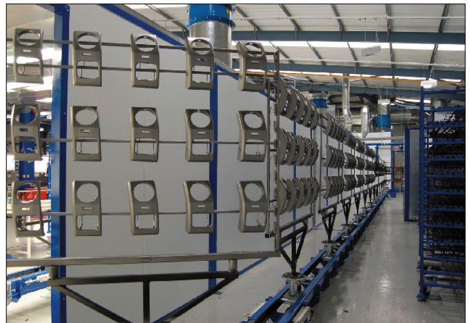
The paint line at M&S Automotive Coatings is based on a 121-metre long Caldan 'HD 100' floor conveyor system, which provides highly accurate positioning of the paint jigs and can operate on a batch "stop-go" or continuous basis, depending on production requirements. A floor-based system was selected in preference to an overhead conveyor as it minimises the risk of contamination of the parts — when coating plastics, optimum cleanliness is of paramount importance. Extremely stable and low in noise, the conveyor has a load capacity of up to 400kg per wagon and operates in temperatures of up to 250...C. It includes automatic lubrication to ensure smooth running, and also has the adaptability to be converted to power-and-free operation.
